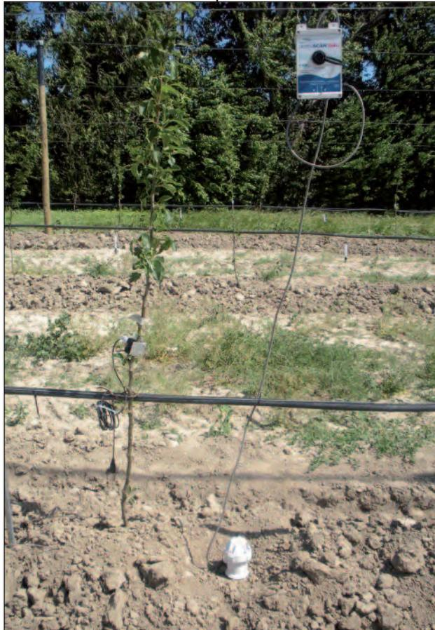
**The tensiometric measurements are particularly useful for detecting any unusual, but not uncommon, incidents or mishaps: difference in the soil types, plough pans causing waterlogging...**
