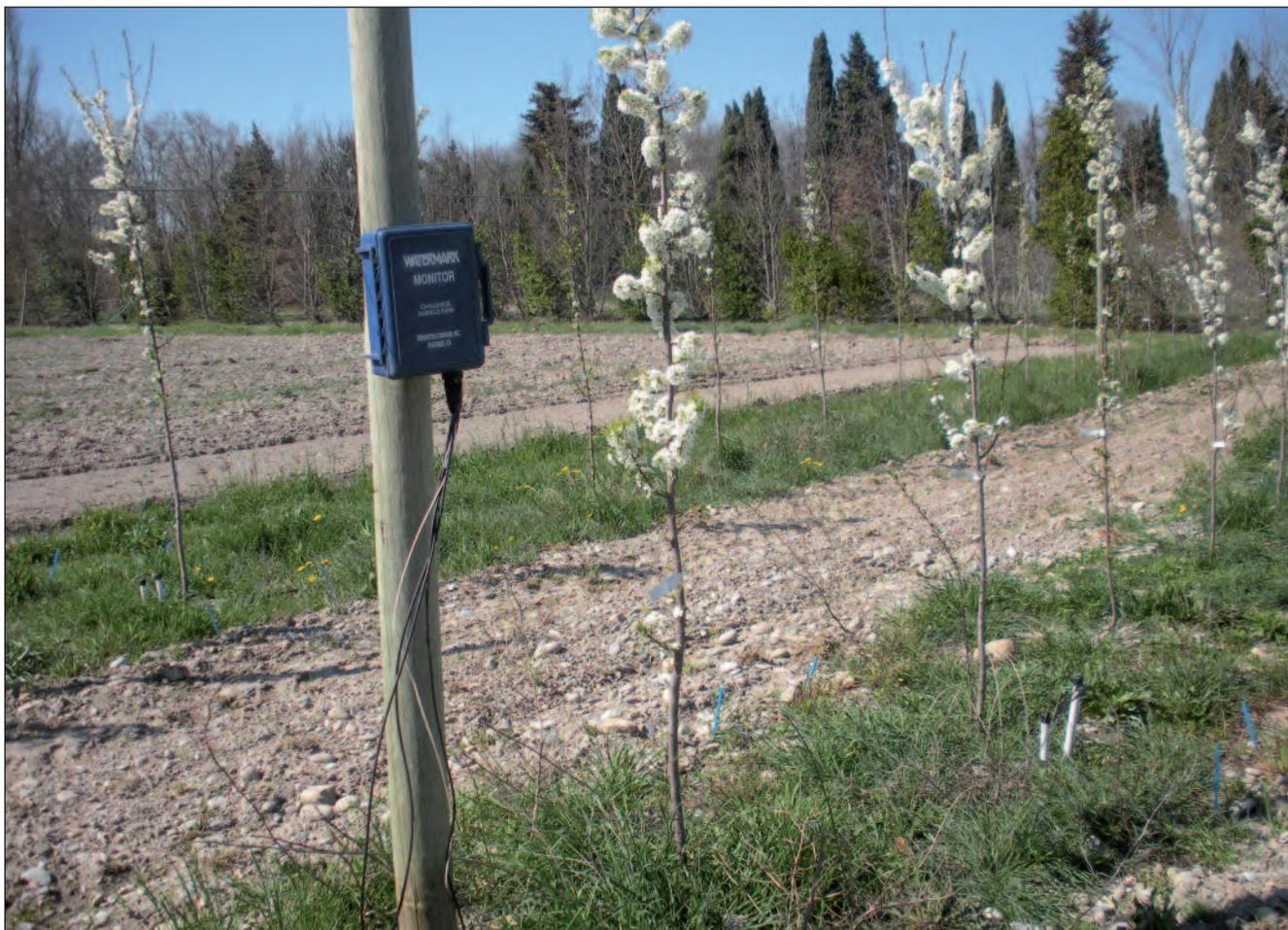
**TENSIOMETRY, WHICH SHOWS HOW MUCH SUCTION IS REQUIRED TO WITHDRAW WATER FROM THE SOIL, GIVES US A DIRECT INDICATION OF HOW MUCH SOIL WATER IS READILY AVAILABLE TO THE ROOTS.**
